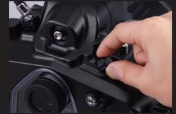
When the focus/zoom dial is pulled out, the gear inside the housing will move outward allowing for lenses with large diameters to be easily mounted.
