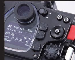
Equipped with two fiber-optic cable sockets. With the camera's built-in flash raised and fiber-optic cables fitted, external strobes can be triggered as "slave units" by the built-in flash.
